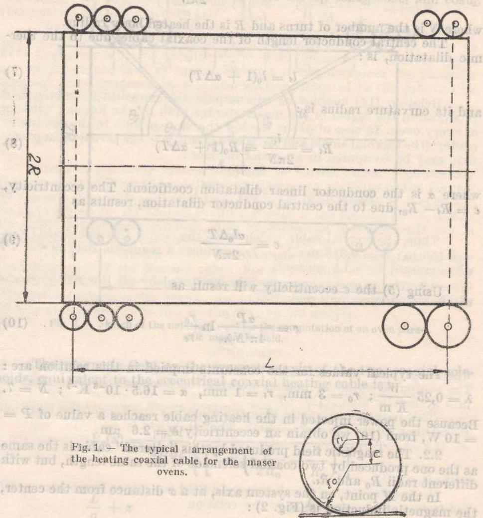
Fig. 1. — The typical arrangement of the heating coaxial cable, for the maser ovens.
